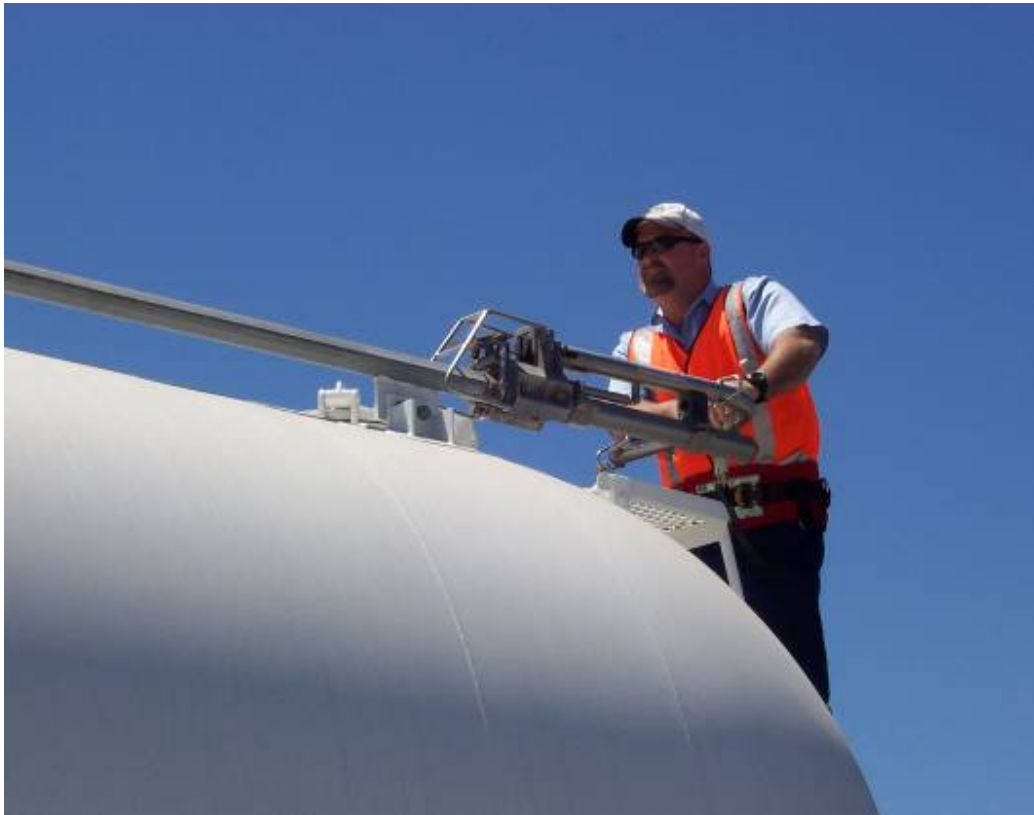
Figure 3 – The TRAM positioned at the rear of the tanker allowing easy access for the operator to connect his safety belt to the attachment points on the TRAM Arm.
